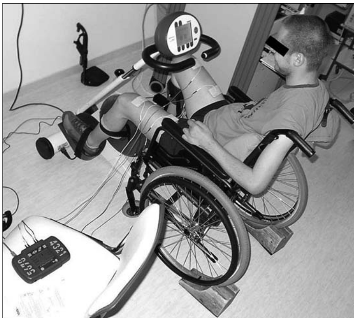
Figure 3. Functional electrical stimulation cycling measurement setup. Stimulator, electrodes with a patient, who is cycling on an ergometer
